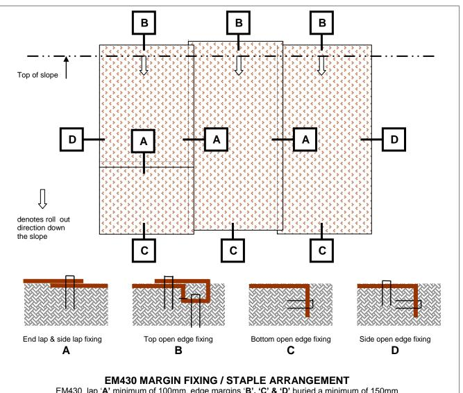
EM430 lap '**A**' minimum of 100mm, edge margins '**B**', '**C**' & '**D**' buried a minimum of 150mm Side laps arranged 'shingle fashion' away from prevailing wind
