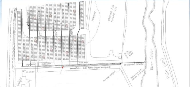
Figure 1. Plan of Lochwinnoch Cemetery including Flo-Pipe and Atlantis Matrix Tank modules
