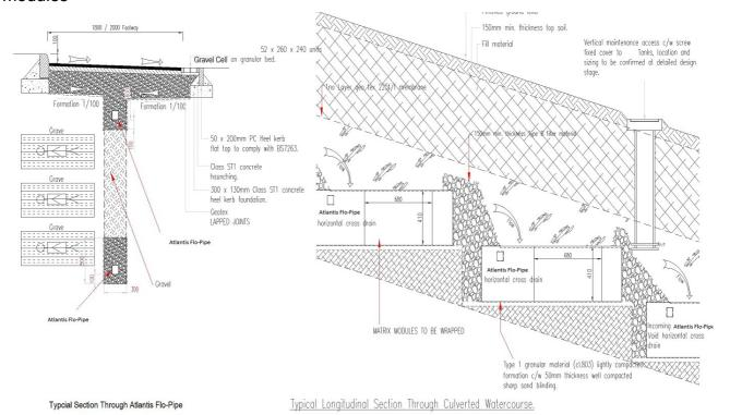
Figure 2. Cross-section showing Flo-Pipe and Atlantis Matrix Tank modules
